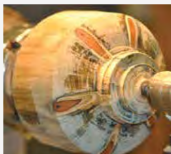
I mounted a turning blank between centers, using a Oneway Big Bite drive and a live center in the tailstock. With the lathe set at a slow speed, I trued the cylinder using a spindle-roughing gouge.
