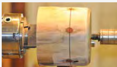
I mounted a turning blank between centers, using a Oneway Big Bite drive and a live center in the tailstock. With the lathe set at a slow speed, I trued the cylinder using a spindle-roughing gouge.
