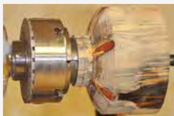
I remounted the cylinder into a four-jaw chuck so that the base of the mushroom was toward the tailstock, and began shaping the stem.
