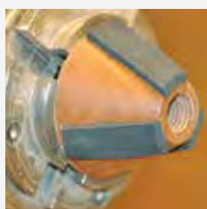
To finish the mushroom, I reversed the piece again and used a cone chuck with pressure from the tailstock. After reducing the tenon to a small nubbin, I carefully parted it off and sanded the top. The toadstool was ready for finish.
