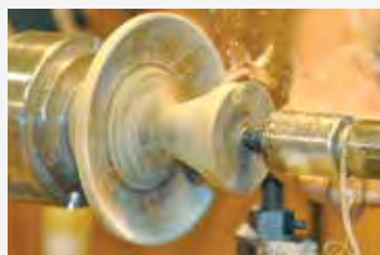
I remounted the cylinder into a four-jaw chuck so that the base of the mushroom was toward the tailstock, and began shaping the stem.
