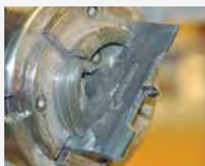
I mounted a turning blank between centers, using a Oneway Big Bite drive and a live center in the tailstock. With the lathe set at a slow speed, I trued the cylinder using a spindle-roughing gouge.
